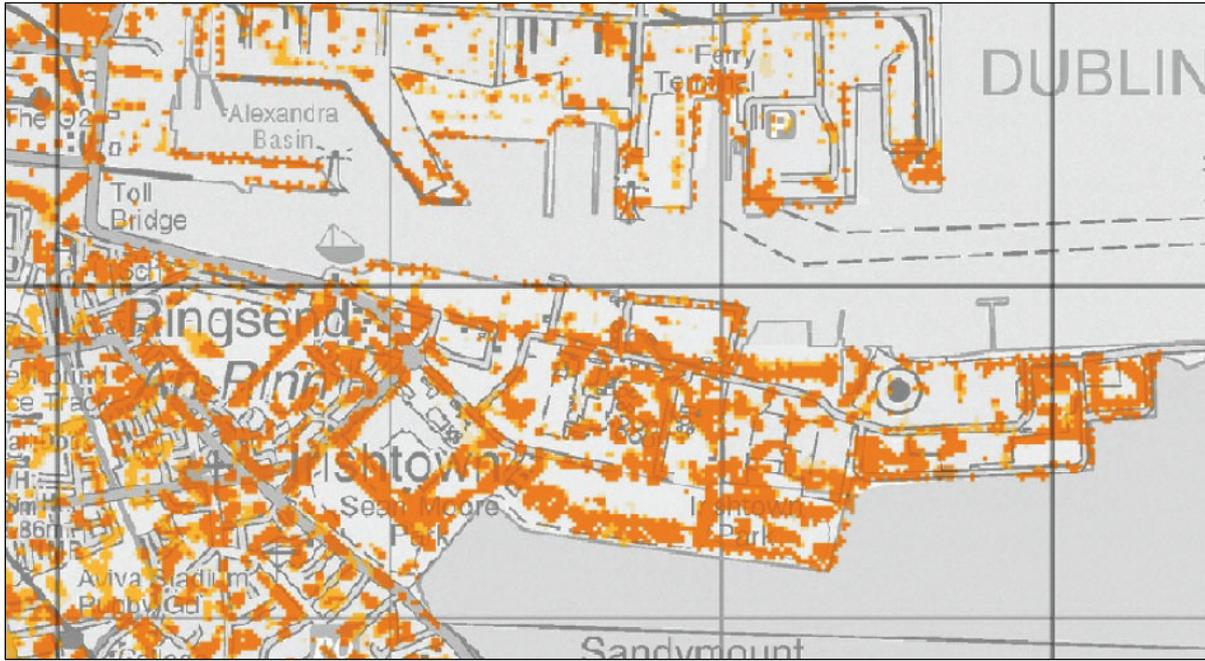
Figure 9-32 Extract from Pluvial Flood Extent Map (Dublin Pluvial Study)
